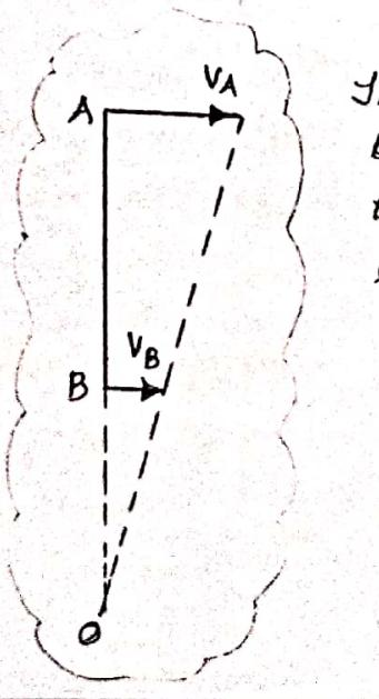
In this case the instantaneous centre will be the point of intersection of line joining the tip of the velocity vectors and the extension of the line joining the points.
