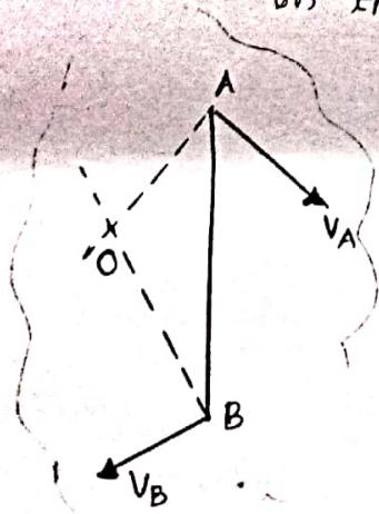
In this case, the instantaneous centre will be the point of intersection of the lines drawn perpendicular to the direction of velocities.
