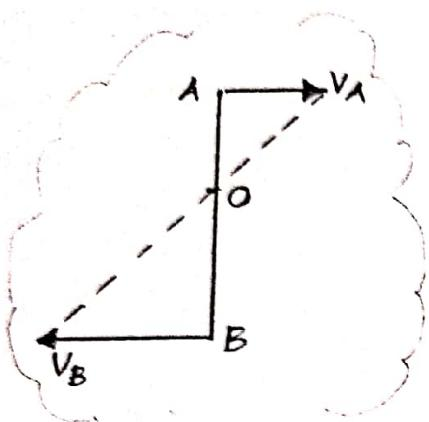
In this case, the instantaneous centre will be the point of intersection of the line joining the tip of the velocity vectors and the line joining the points.
